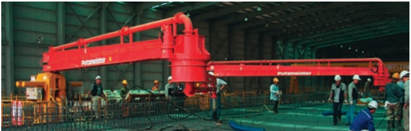
RV 16 rotary distributor in use in the production of bridge sections
